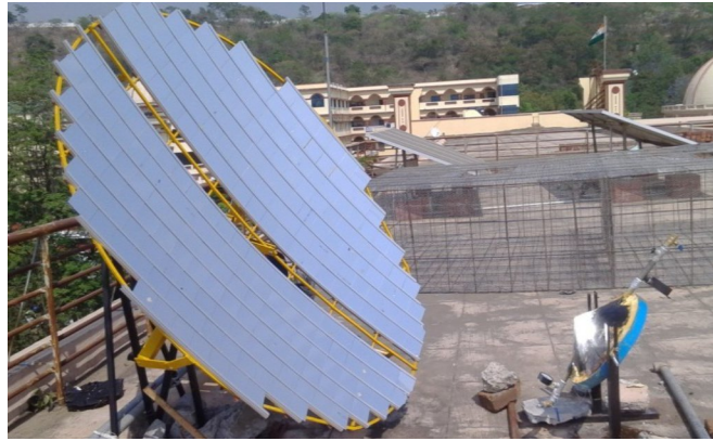
Figure 2.2: Small Scheffler with conical receiver
