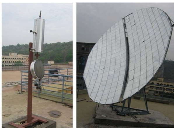
Figure 2.1: Big Scheffler with cylindrical receiver
