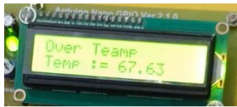
Figure 5. Over temperature fault detection on LCD display
