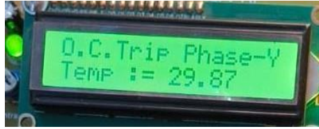
Figure 4. Over current fault detection on LCD display
