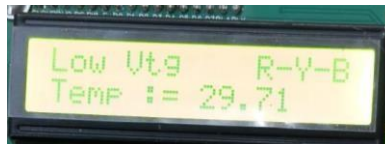
Figure 6. Under voltage fault detection on LCD display
