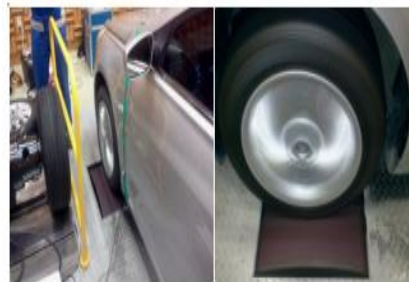
Figure 6.3.1 rolling cleat test to measure the sound pressure in a vehicle
