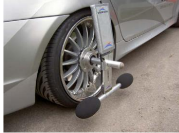
Figure 6.2.1 – CPX measurement set-up
