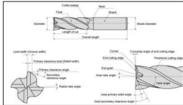
Fig. 1. End milling cutter
