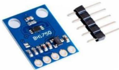
Fig.5 -BH1750 digital ambient light sensor
