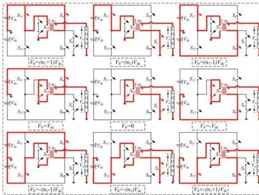
Figure 2: Modes of operation of the proposed inverter topology
