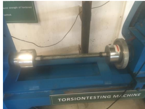
Fig.11 Shaft attached for testing on torsion testing machine.
