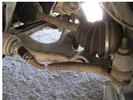
Fig.2 Image of a broken tie rod
