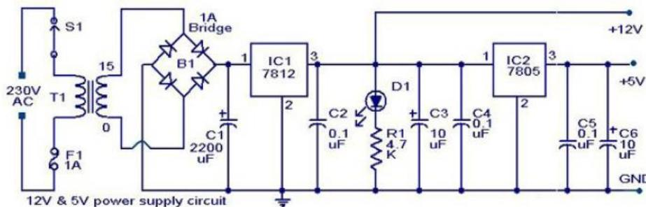
Fig 3.1 Power Supply Circuit Diagram
