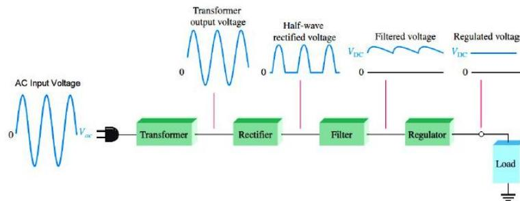
Fig 3.2 Working Principle of Power Supply
