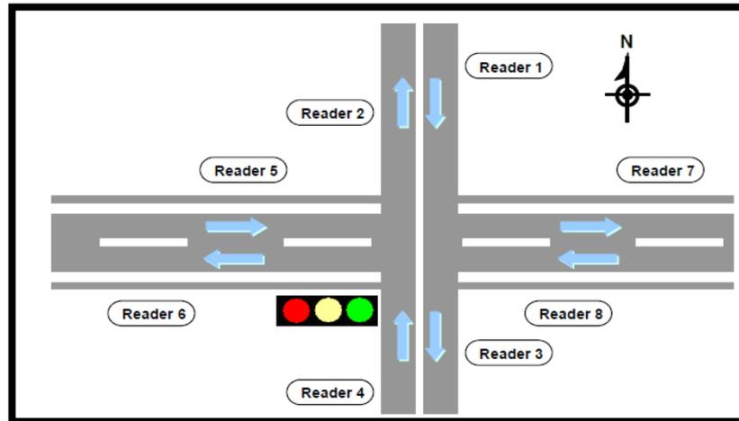
Fig 3 – Placement of RFID readers at strategic locations across signal
