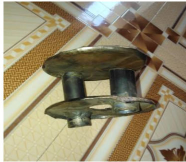
Fig No.5.1.1 PART SECOND (turning chamber)
