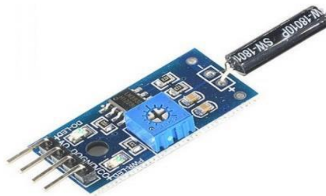
Fig -vibration sensor
