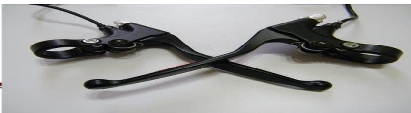
The e-brake lever is a replacement for the regular brake lever and either cuts out the controller or engages regenerative braking in the controller when the lever is squeezed. We have integrated levers for both mechanical and hydraulic brakes, as well as a TripWire product which can be added to your existing levers to turn them into e-brakes. All operate as a NO switch, with two wires that close the circuit when the brakes are engaged.
