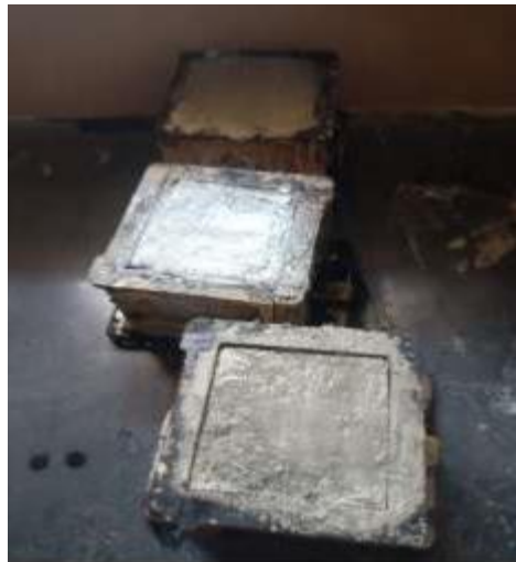
Fig.No.1 Casting of blocks and setting
