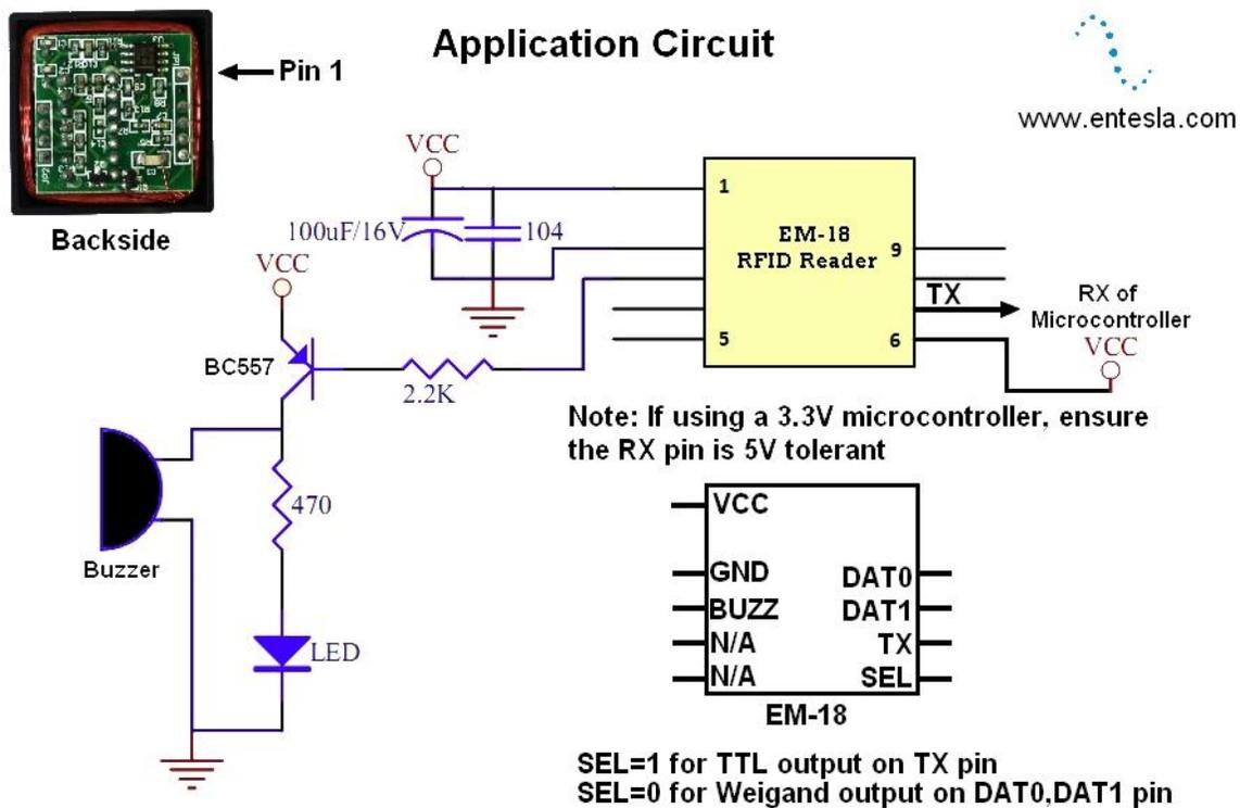
Fig 6- Application circuit of RFID tag reader
