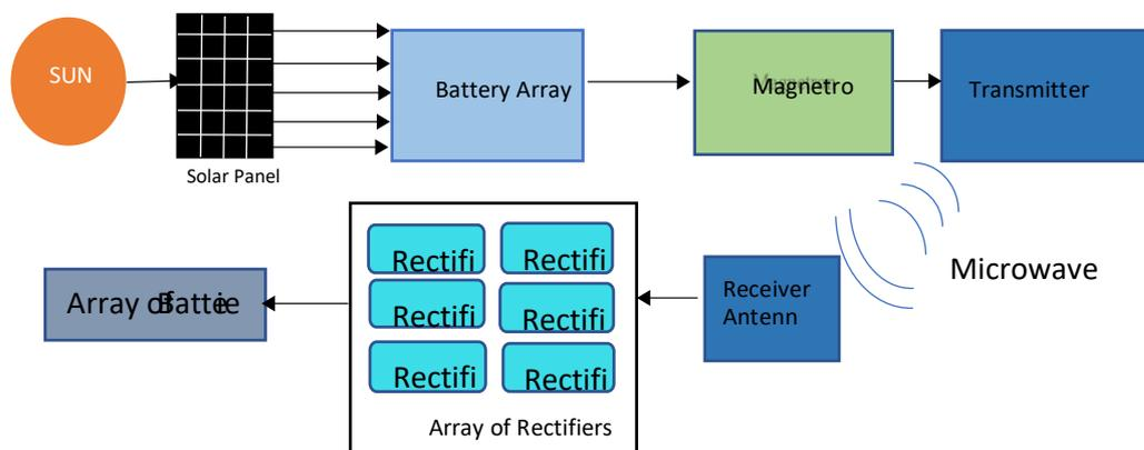
Fig.1 Block diagram of proposed SSP
