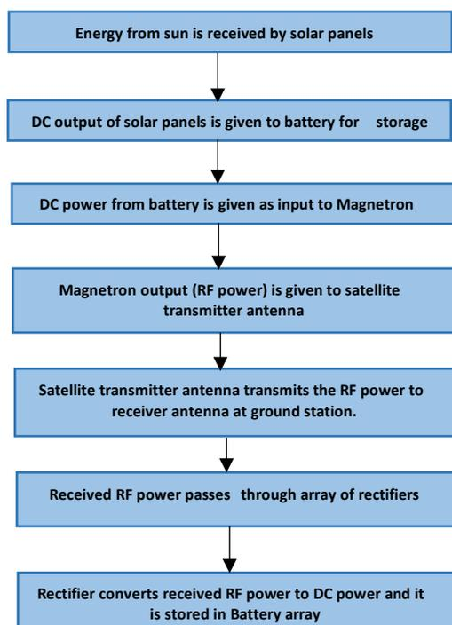
Fig.2 Workflow of the Space Solar Power System
