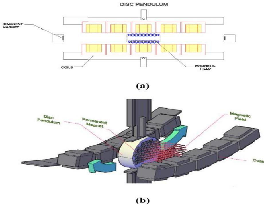
Fig.2: Magnetic Field of Disc Pendulum
