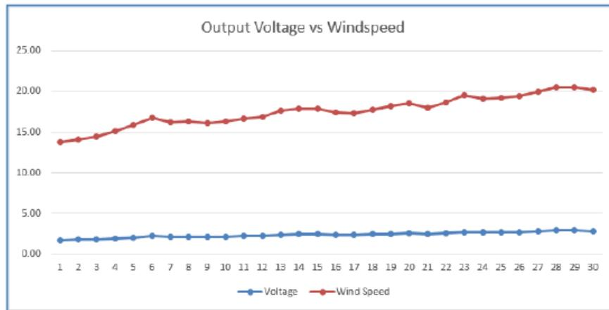
Fig.6: Wind Speed vs. Voltage Graph of the multi-directional pendulum
