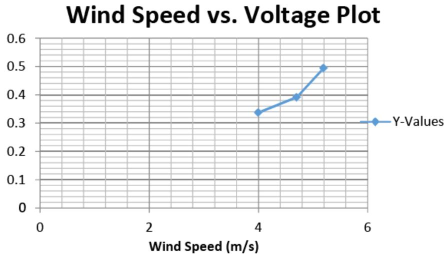
Fig.5: Wind Speed vs. Voltage Graph of the Disc shaped pendulum
