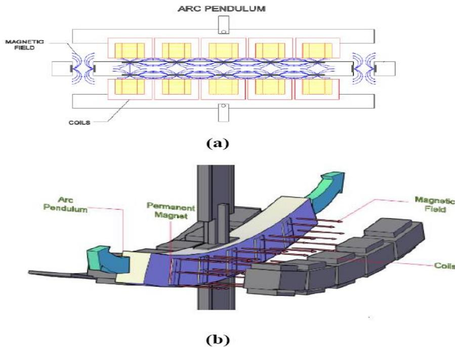
Fig.1: Magnetic Field of Arc Pendulum
