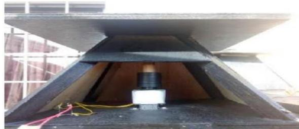
Fig.3: Multi-Directional pendulum
