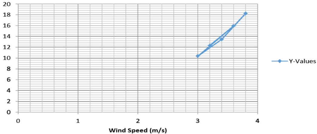
Fig.4: Wind Speed vs. Voltage Graph of the Arc shaped pendulum
