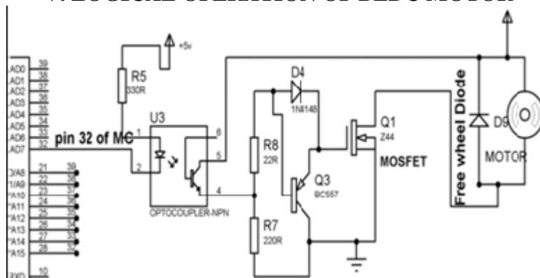
Fig.7 : PWM Generating Circuit
