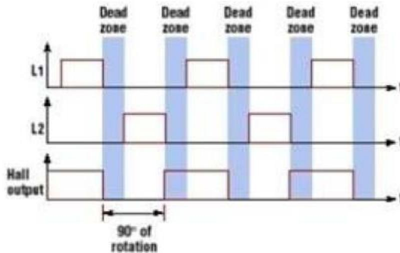
Fig . 3: Commutation Timeline Diagram
