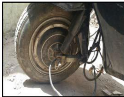
Fig. 2. Side view of the hub motor fitted on the front wheel of the vehicle
