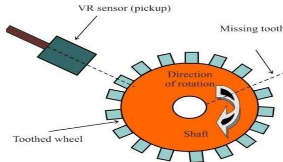
Fig. 3 BLDC motor with VR Speed sensor
