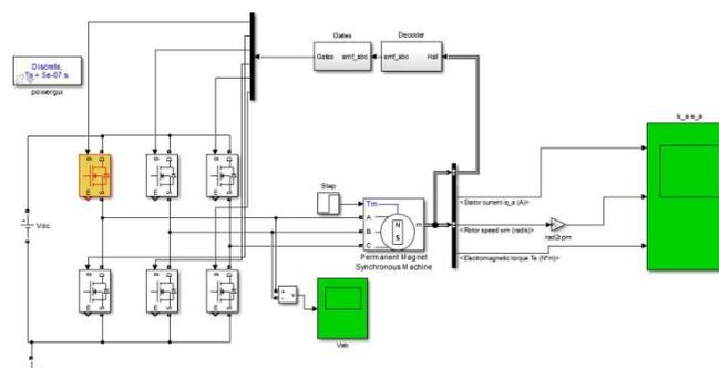
Fig 6 Simulink Motor Model of Proposed System
