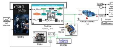
Fig 8 HEV System Level Layout
