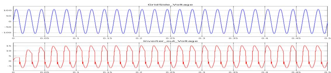
**Fig. 7.** Grid side voltage and inverter out voltage in PV Grid Mode.
