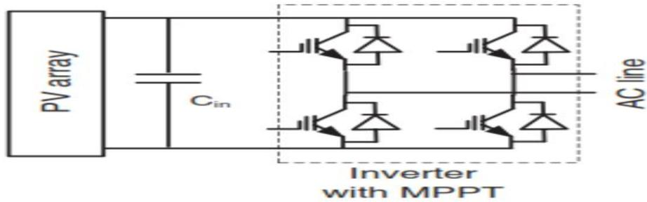
**Fig 5** Full-bridge with MPPT-based circuit topology of single stage inverter
