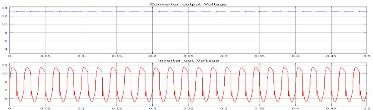
FIG. 10. Converter and Inverter output voltage PV-battery- Grid mode.
