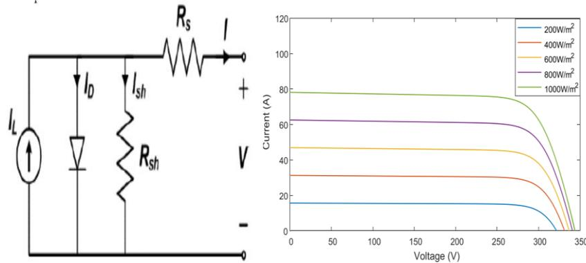
**Fig 2:** Equivalent circuit of PV cell **Fig 3:** I-V characteristics of 20kW PV Array at different irradiation levels
