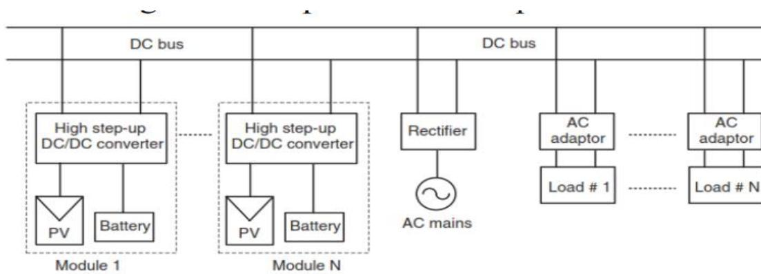
**Fig 4** PV-battery-powered DC bus system
