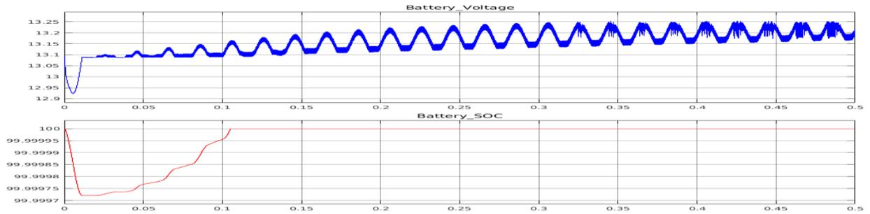
Fig. 12. Battery voltage and battery SOC in PV-battery- Grid mode.
