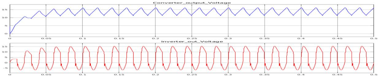
Fig. 8. Converter and Inverter output voltage PV Grid mode
