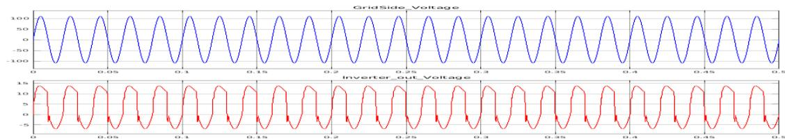
Fig. 9. Grid side and Inverter output voltage PV-battery- Grid mode.
