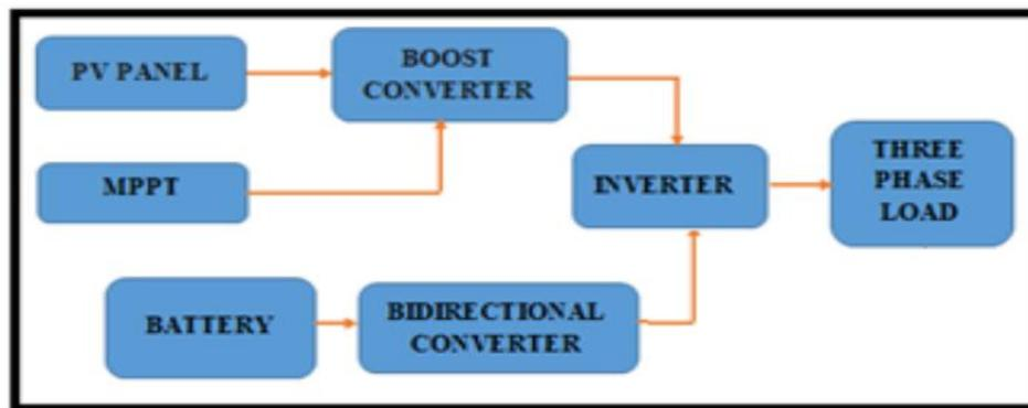
Fig.1 Block Diagram of MPPT Techniques based Photovoltaic System
