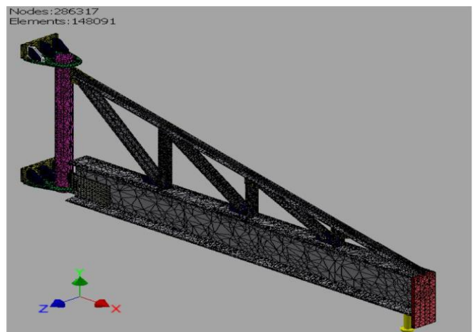
Figure 2. Typical 3-d Model of Wall Mounted Jib crane
