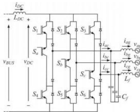
Fig.1. Bidirectional Current Source Converter (CSC)
